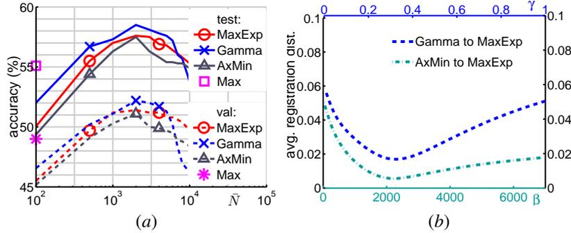
Figure 7: Baseline LcSA mid-level coding (Caltech101, 15 training images/class, no spatial information, linear kernels). (a) LcSA with Max, MaxExp, Gamma, and AxMin pooling. Gamma and AxMin are brought to the MaxExp parameter space  $\bar{N}$  by registration (eq. (20), sec. 3.3). Dashed and solid curves show the validation and test results. (b) Corresponding average registration distance between Gamma/AxMin and MaxExp signatures highlights their closeness.
