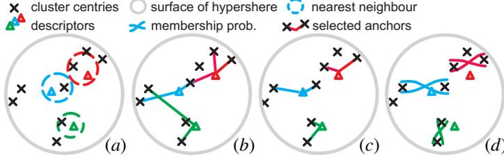
Figure 2: Illustration of (a) Hard Assignment, (b) Sparse Coding, (c) Locality-constrained Linear Coding, (d) Approximate Locality-constrained Soft Assignment. Descriptor vectors (triangles) are scattered on a surface of a hypersphere amongst the anchors (crosses). Note the difference between SC and LLC.
