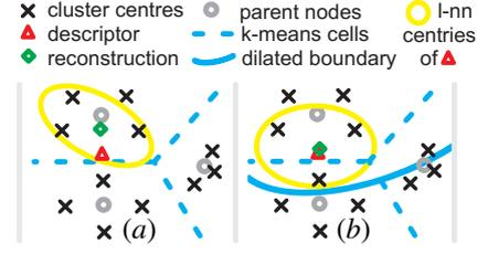
Figure 3: (a) Hierarchical NN:  $l$ -nearest anchors of a descriptor found in its nearest k-means cluster. (b) Dilating cluster boundaries improves quantisation: a descriptor and its reconstruction are brought closer.
