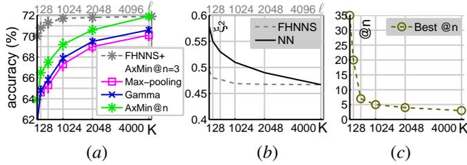
Figure 14: Performance of LcSA given Fast Hierarchical Nearest Neighbour Search (section 2.7) and ordinary NN (Caltech101, 15 training images/class, Spatial Pyramid Matching). (a) LcSA with FHNNS as a function of  $\ell$  (cluster dilation). Also, LcSA with NN as a function of  $K$  (dictionary size) for Max, Gamma, and AxMin@ $n$ . (b) Corresponding quantisation errors  $\xi^2$ . (c) The optimal value @ $n$  for AxMin@ $n$  as a function of the dictionary size  $K$ .
